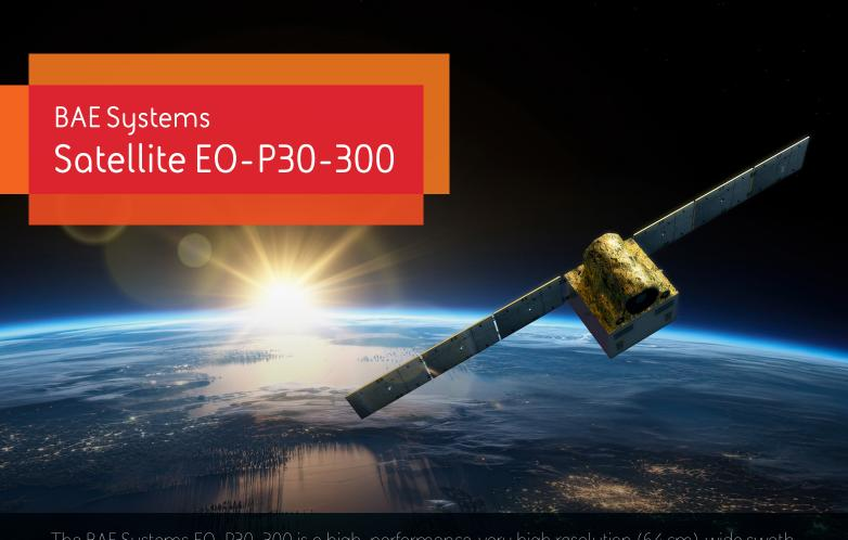
The BAE Systems EO-P30-300 is a high-performance, very high resolution (64 cm), wide swath earth observation small satellite with complimentary full motion video up to 30 frame-persecond. The platform also features an onboard mission processing system and comes with an intersatellite link to support dynamic tasking.
